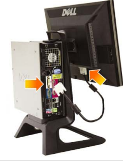
4 Connect the white DVI cable to the computer
