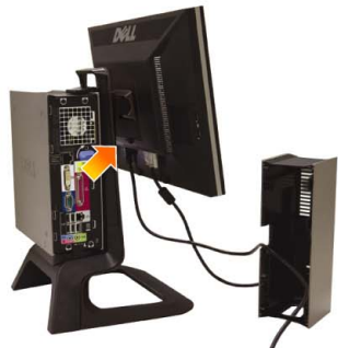
5 Connect the power cable to the monitor as shown
