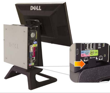
2 Slide the computer onto the stand
