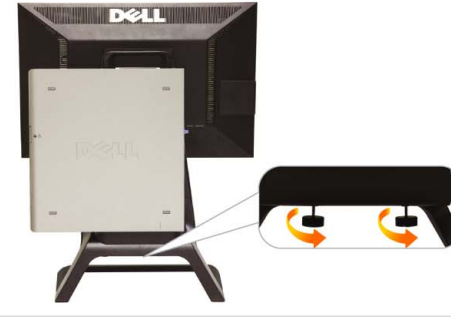
3 Tighten the screws underneath the stand
